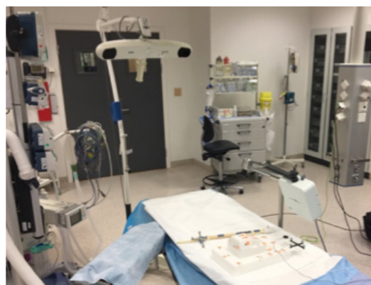
OR setup with the optical and the electromagnetic tracking systems Picture: The Intervention Center and SINTEF
