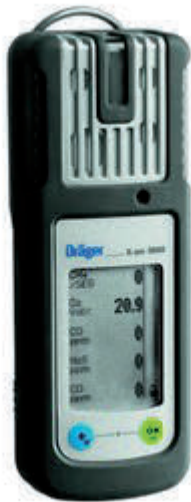
Figur 27 Dräger X-am 5000 gassmåler
