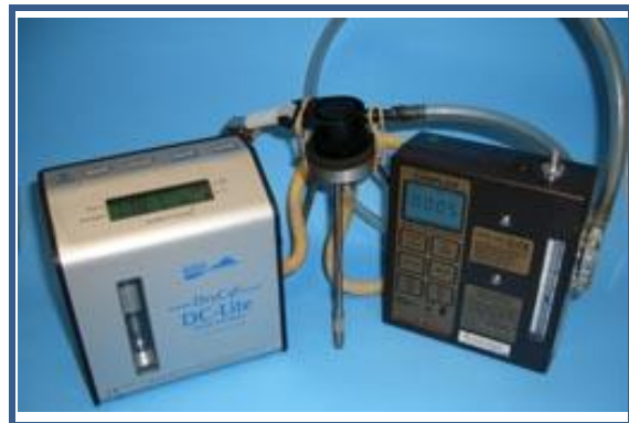
Figure 5-21 Calibration with Electronic Flow Meter
