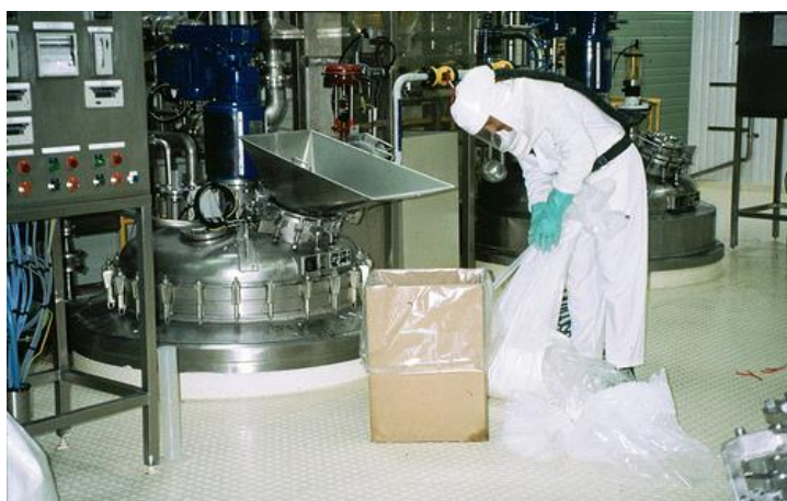
Figure 10.10 – Addition of sack of powder to reactor
