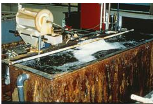
Figure 9.9 – Electroplating bath with detergent foam
