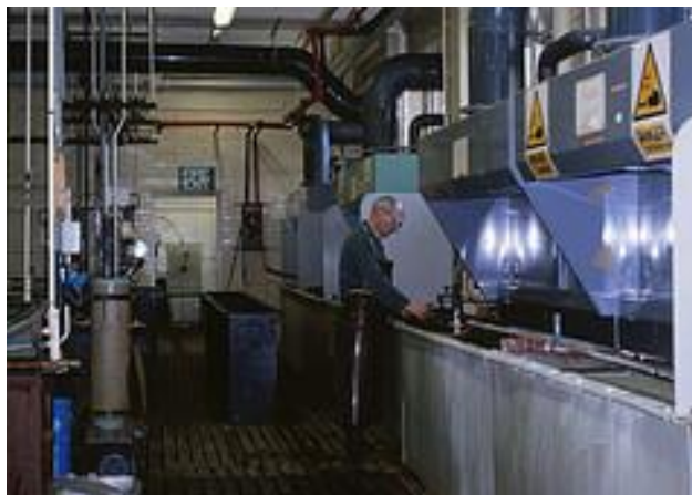
Figure 9.10 – Electroplating bath fitted with local exhaust ventilation
