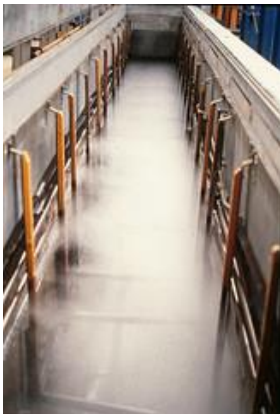
Figure 9.14 – Large vapour degreasing tank fitted with cooling coils and slot extraction at the rim
