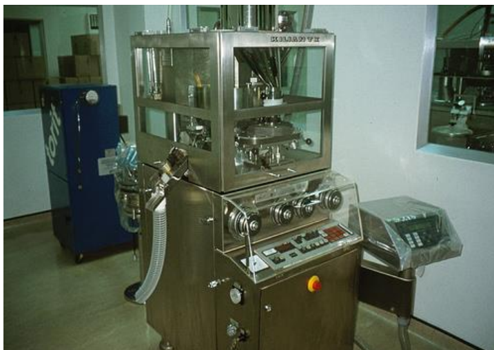
Figure 10.11 – Fully enclosed tablet press with extraction
