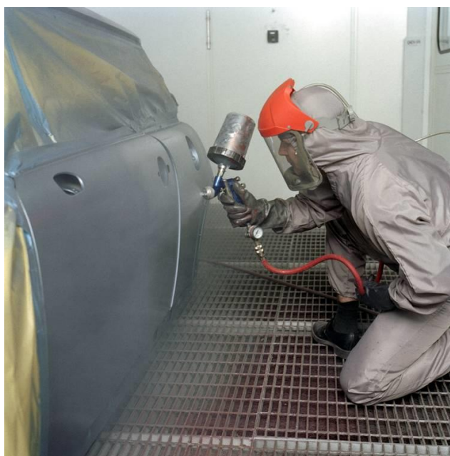
(Source: HSE LEV Trainer Adviser Briefing Days – reproduced with permission) Figure 9.15 – Spraying isocyanate based paint in paint spray booth
