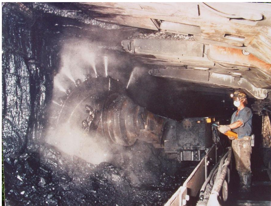
Figure 10.9 – Longwall coal mining with water sprays
