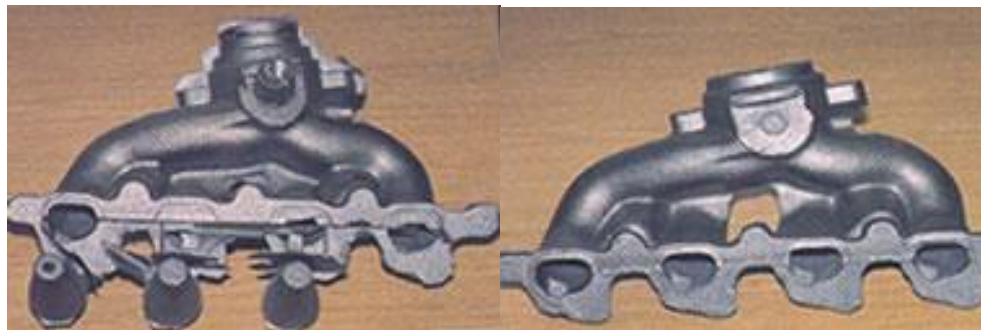
Figure 10.5 – Casting before and after fettling
