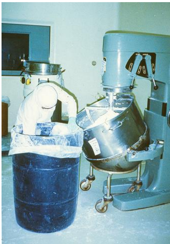
Figure 9.2 – Manual loading of open mixer from drum
